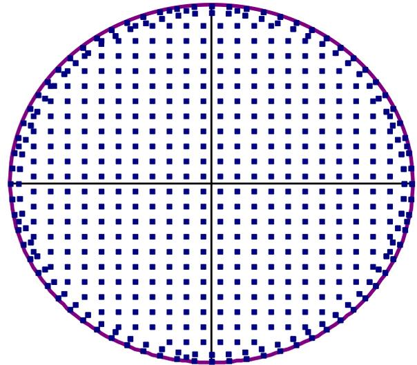
Fig. 19 Plan view and pile layout of the simulated hypothetical tank
