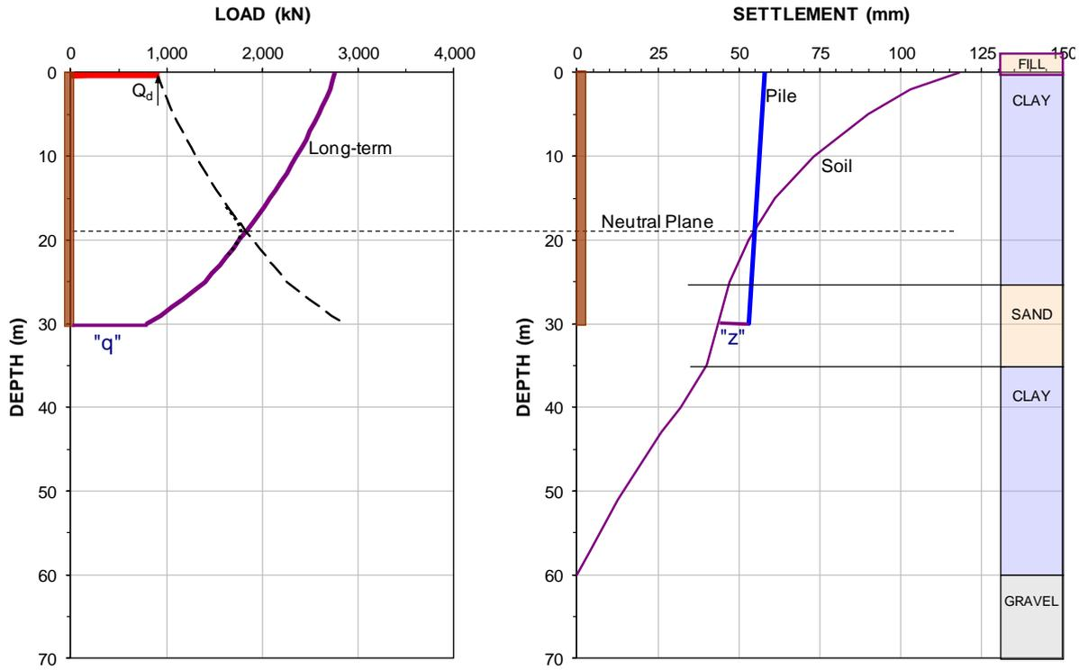
Fig. 22 Load and resistance distribution supplemented with settlement distribution
