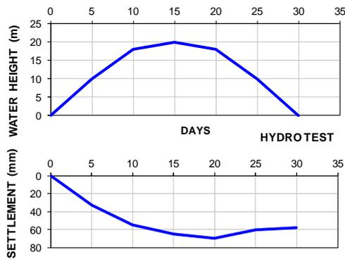
Fig. 23 Simulated settlement response for an assumed hydrotest
