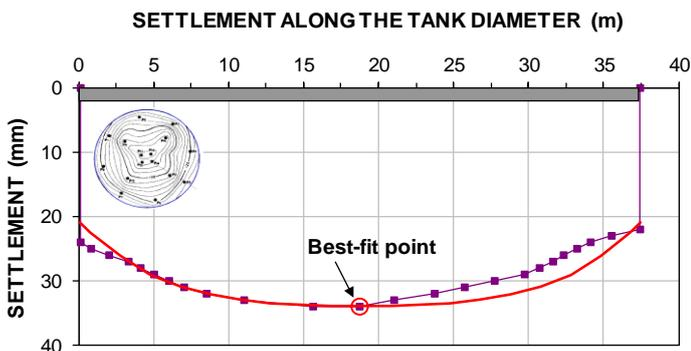
Fig. 18 Measured and calculated settlements for the Thessaloniki hydro tested tank
